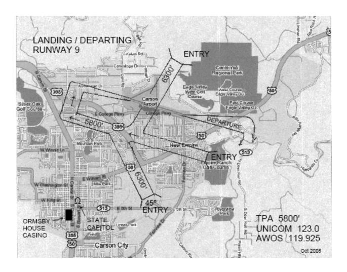
When using runway 9, except as safety dictates otherwise, all aircraft taking off must proceed straight ahead until reaching the end of the runway and execute a slight left turn to 85 degrees. After attaining a minimum altitude of 700 feet AGL (5400 feet MSL) and ascertaining there is no danger of collision with other aircraft, resume normal navigational procedures.
