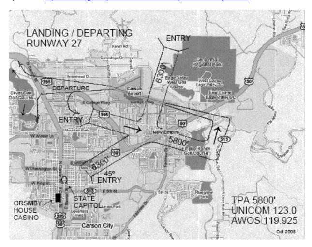
When using runway 27, except as safety dictates otherwise, all aircraft taking off must proceed straight ahead until reaching the end of the runway and execute a left turn to a heading of 230 degrees as soon as safely possible. After attaining a minimum altitude of 700 feet AGL (5400 feet MSL) and ascertaining there is no danger of collision with other aircraft, the pilot may execute a left or right cross-wind turn as appropriate.
